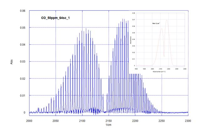
Examples of CO spectrum measured with GASEX HD-05-12 in comparison to the GASEX ST-20-12 with 2 cm<sup>-1</sup> (inset of the picture) resolution.
