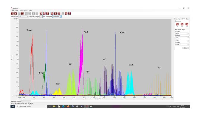
Examples of various gases spectra measured using using a GASEX HD-05-12 (screenshot) shorwing a variety of substances measured, within the 2-12 micons range or operation of these spectrometers.
