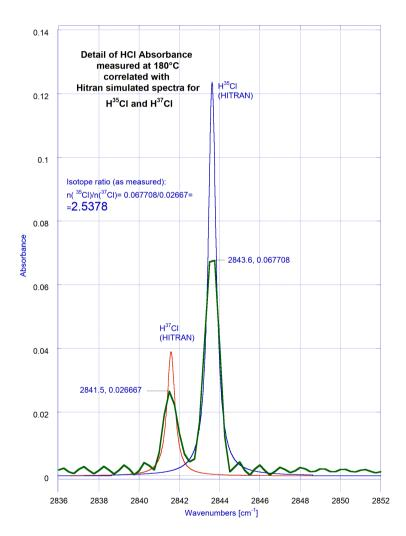
Examples of HCl measurments using a GASEX HD-05-12 together with HITRAN simulation of the spectra for HCl with <sup>35</sup>Cl and <sup>37</sup>Cl isotopes in the molecule. The isotope ratio can be determined.
