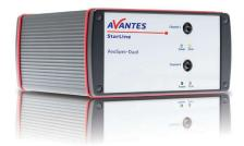
Sometimes a single channel spectrometer is not enough, for example when you want higher resolution or to do two redundant measurements at the same time. The AvaSpec dual channel spectrometers are designed specifically for this purpose. Each spectrometer can be configured independently. It is also possible to have different detector types in each channel.
