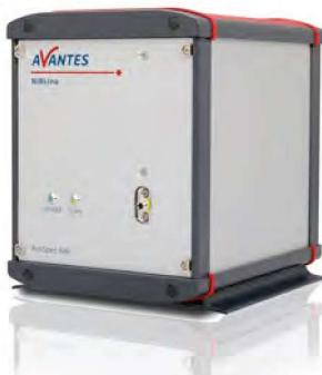
The new and improved versions of our NIR spectrometers offer more sensitivity, less weight and less size. They are based on a 100mm optical bench with a NA of 0.13 offering optimal balance between resolution and sensitivity.
