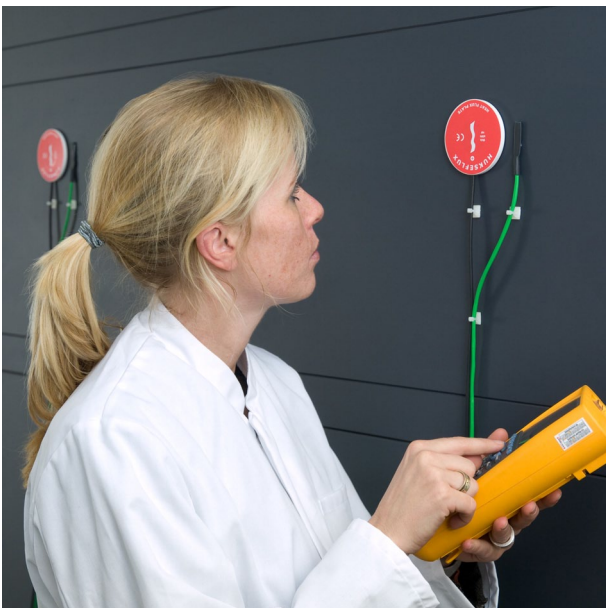
Figure 2 HFP01 heat flux sensor in use
