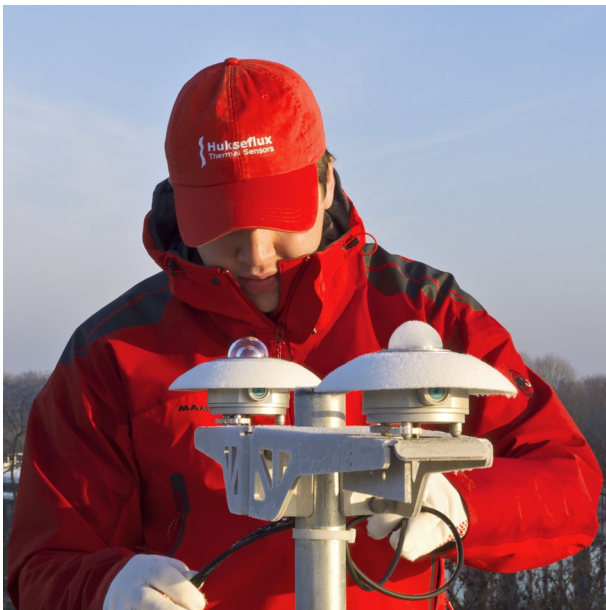
Figure 2 frost deposition: clear difference between SR25-D2 (left), versus a non-heated pyranometer without sapphire dome (right)
