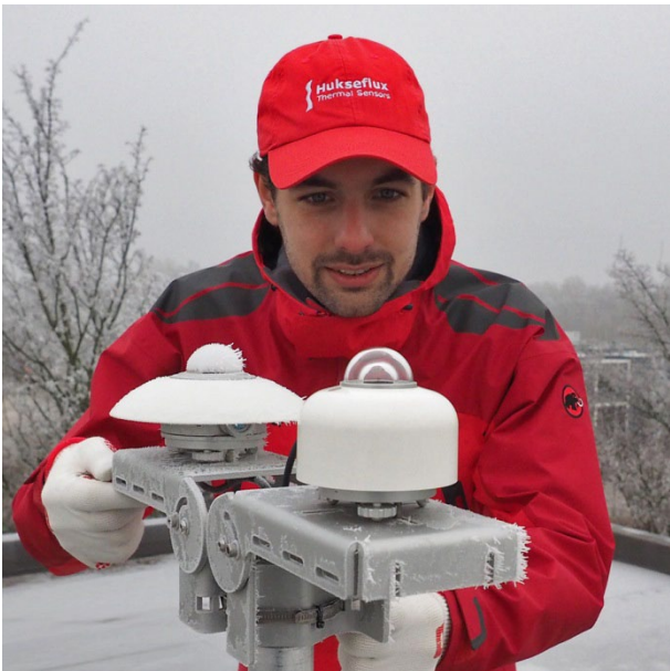
Figure 3 frost and dew deposition: clear difference between a non-heated pyranometer (back) and SR30 with RVH™ technology (front)
