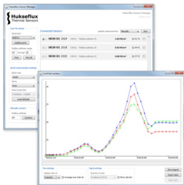
Figure 5 user interface of the Sensor Manager, showing sensor diagnostics
