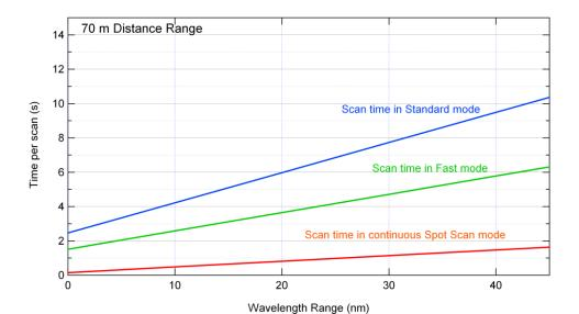
Time per scan vs. scan wavelength range for 70 m scans in standard operating, fast scanning and continuous spot scanning modes.
