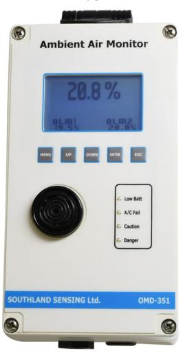
The OMD-351-O2 Ambient Air Monitor is designed to measure and assure the appropriate level of oxygen in an enclosed or confined area. Personal safety is a primary issue in nearly every industry and is magnified within confined spaces where oxygen depletion or asphyxiation due to a leak in an inert gas container can quickly and unexpectedly take place.
