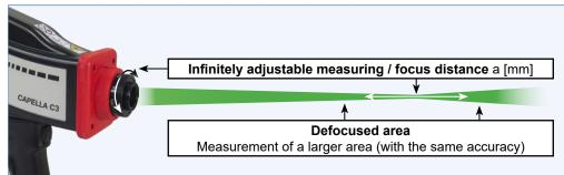
Measuring / focus distance a [mm] (all intermediate values adjustable)
