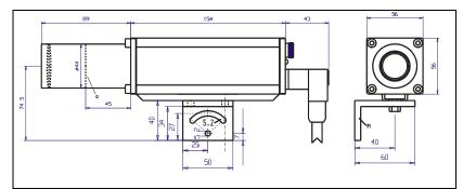
Depending on type, length of lens tube is either 45 mm or 89 mm.
