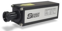
developed. Furthermore it is best choice to measure thin glass surfaces in furnaces because glass is neither transparent nor reflective at 8,05 µm. It meets therefore the so called black body conditions of an ideal radiator.
