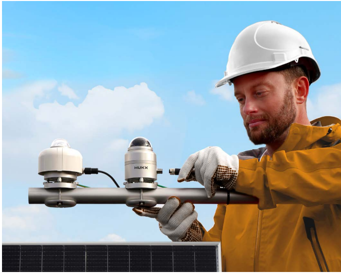
Figure 3 Typical installation of SRD100, next to a normal Class A pyranometer, such as the SR300-D1.
