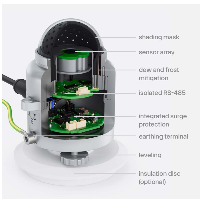
Figure 2 Inside the SRD100 diffusometer: a detailed look at the core components responsible for performance and durability under extreme conditions.
