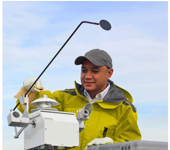
Figure 5 A traditional solution for diffuse and direct solar radiation measurement: an automated, motor-driven dual-axis solar tracker equipped with a pyrhemeter and shaded pyranometer. SRD100 offers a low-maintenance and more robust (no-moving parts) alternative.
